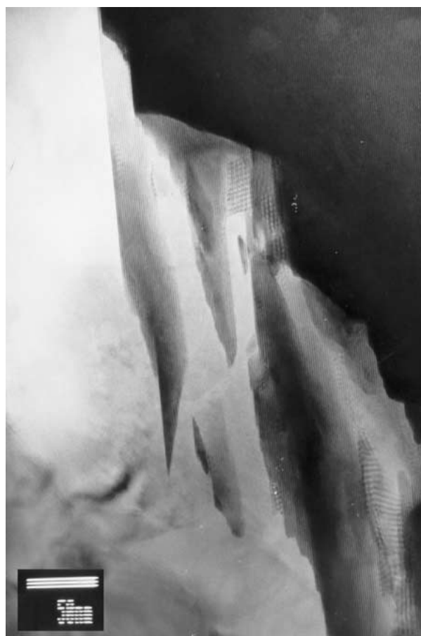
Figure 4 Preferential dissolution of the SiC planes by reaction with the Al-Si-O phase after consumption of the \text{SiO}_2 active barrier.
